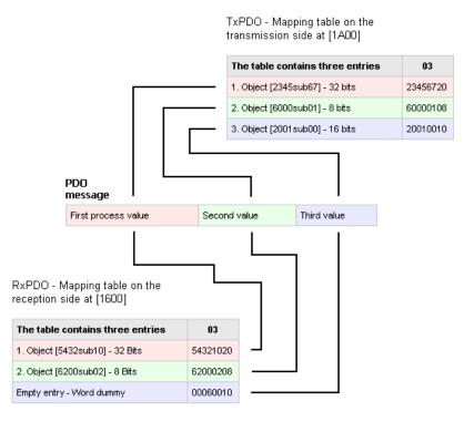
In this example there are exactly two object links: from object (process variable) [2345sub67] of the PDO producer to object [5432sub10] of the PDO consumer and from object [6000sub01] of the producer to object [6200sub02] of the consumer. The third transmit object, [2001sub00] is not evaluated on the receiver side and is therefore covered up with a so-called dummy object.
